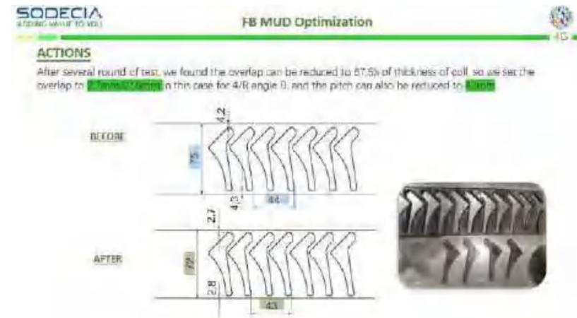
During the production of the 4/R angle in the FB process, we identified a MUD of 41%, resulting in a waste of around 59% of the material. This situation was repeated in all other parts of the FB, generating waste material. We started an analysis and carried out tests to address this issue.
