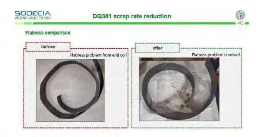
We implemented corrective measures, resulting in a significant reduction in 37's scrap rate.
